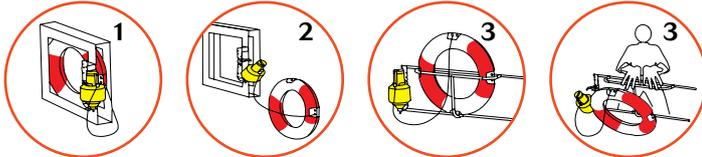
1. Signal and lifebuoy mounted on bridge wing in ready to fire position.
